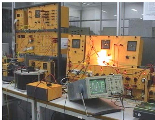
Fig. 16: Three-phase inverter prototype.
