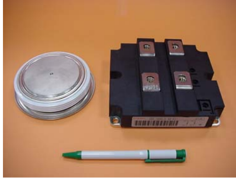
4500V/800A press pack and 1700V/1200A module diodes
